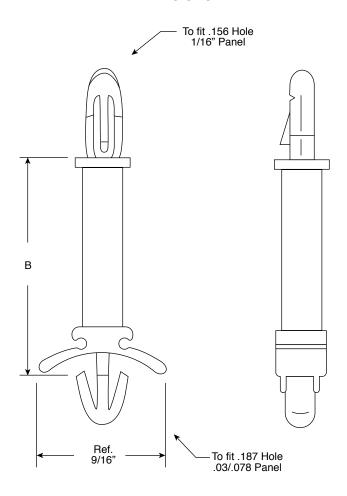
Circuit Board Supports eliminate screws, nuts, and lockwashers in mounting printed circuit boards on metal chassis or stacking in multiple tiers. Unique locking designs provide mechanically secure, reusable connection in predrilled or punched holes while saving considerable assembly time and expense.
